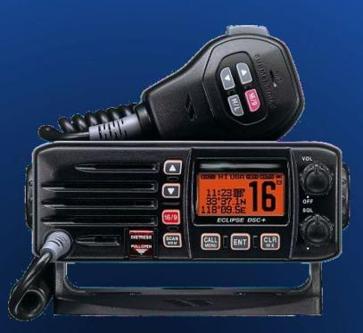
Identifiable by a red button marked "Distress", and "DSC" on the face plate
