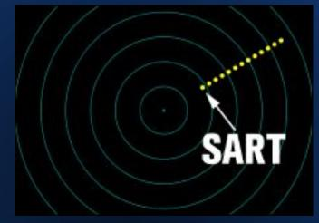
In passive mode batteries last 96 hours – can actively respond to radar signal for 8 hours
